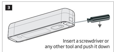
2. Remove the PCB (printed-circuit-board) from the enclosure.
