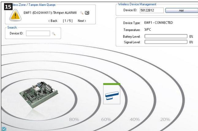
13. Upon the successful binding process, EWD2 device icon becomes visible in **Wireless Device Management** section as well as **Battery Level** and **Signal Level**. If the attempt to bind is unsuccessful, try to move EWD2 closer to the ELDES alarm system and bind anew.
